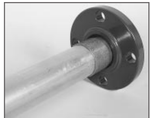
3. Slide the flange back over adapter, align bolt holes, and tighten
